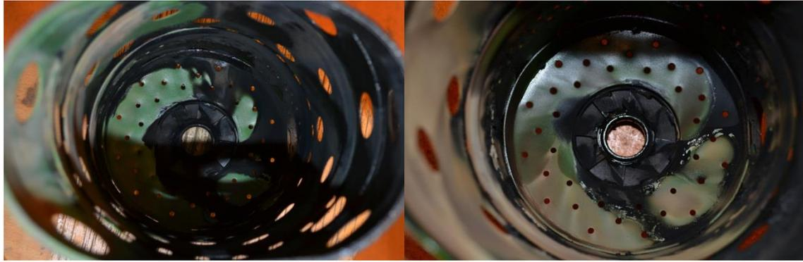
**Figure 8. Combustion chamber before (left) and after (right) the test campaign**
