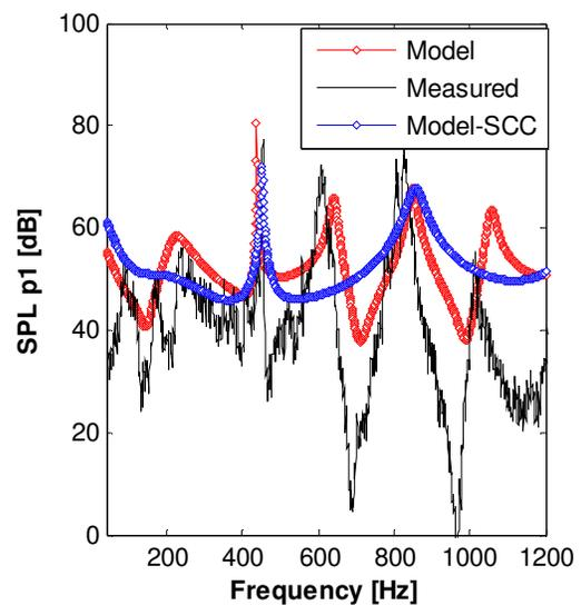
**Figure 9:** Simulation of different length of combustion chamber (SCC is short combustion chamber)
