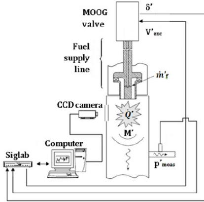
Figure 3: FTF measurement system overview.
