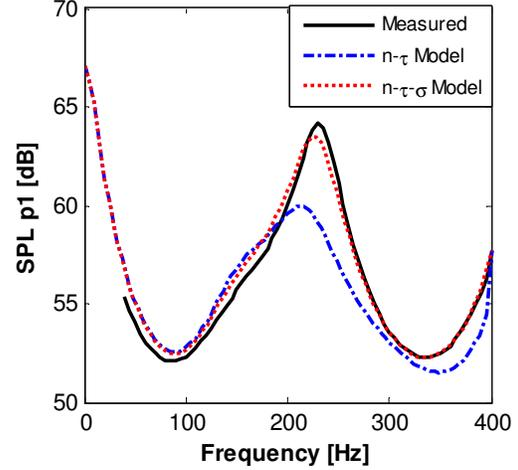
Figure 5: Measured and modeled FTF
