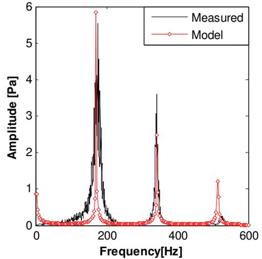
Figure 2: Validation of acoustic network model, impedance tube test
