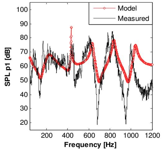
**Figure 8:** Comparison of measured and simulated pressure spectra at location of P1 for 30.5 case
