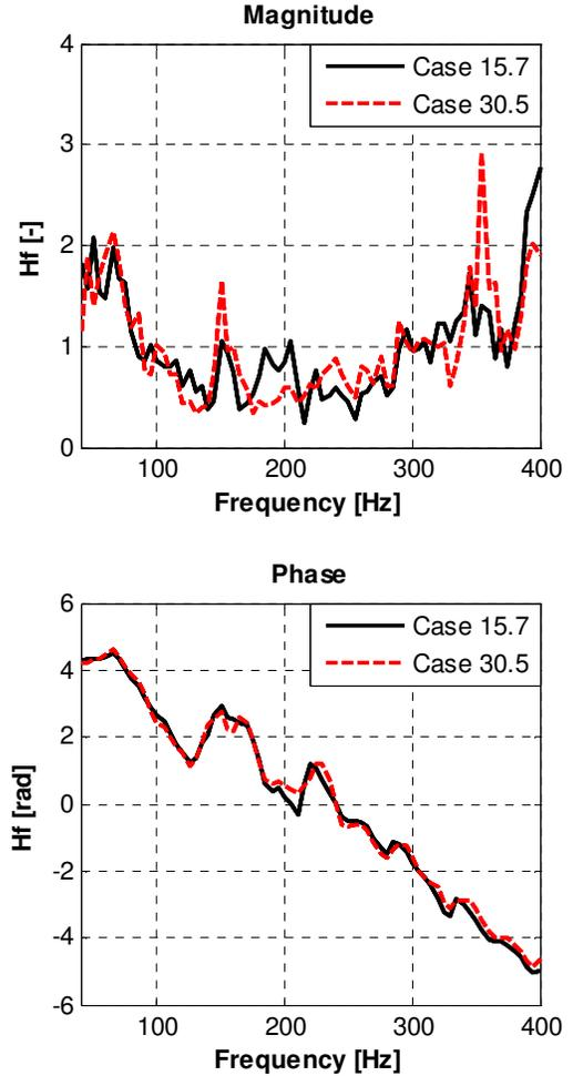
Figure 4: Flame transfer function of the Desire setup
