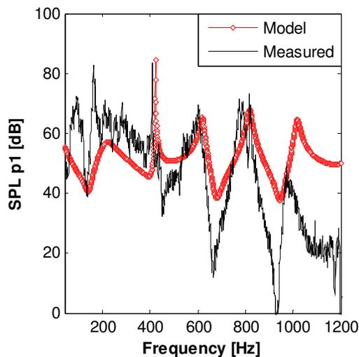
**Figure 7:** Comparison of measured and simulated pressure spectra at location of P1 for 15.7\_2 case
