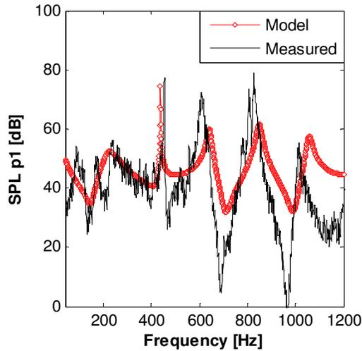
**Figure 6:** Comparison of measured and simulated pressure spectra at location of P1 for 15.7\_1 case
