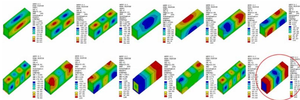
Fig. 2. Results of modal analysis, mode in red circle is the synchronise mode at frequency 176 Hz
