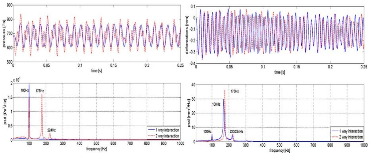
Fig.1. Pressure (left) and deformation (right) pattern during one- and two-way analysis
