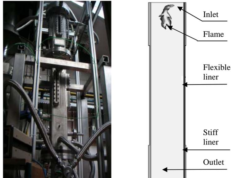
Figure 1. Experimental setup (left) and sketch of the liner geometry (right)
