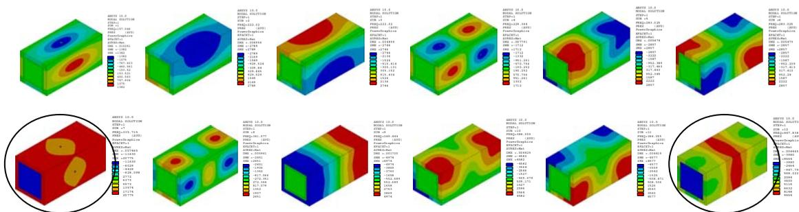
Fig.7. Eigenmodes of the fluid-structure system, synchronised modes are in the circle
