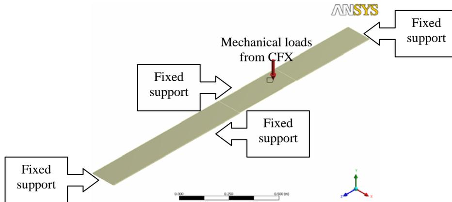
Figure 3. Boundary conditions used for structural analysis
