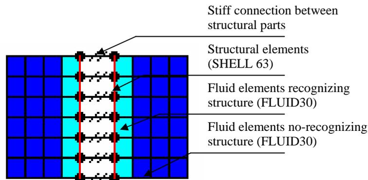
Figure 4. Connection between different elements during modal analysis
