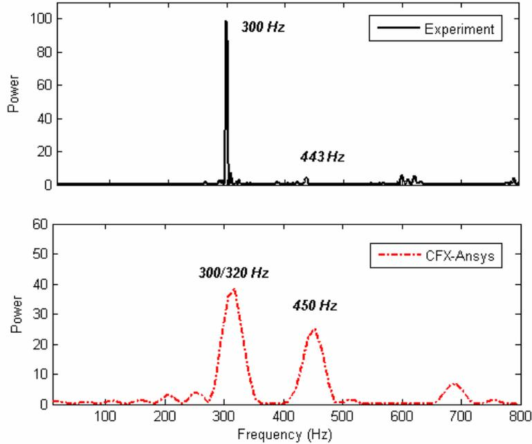
Fig. 6. FFT of the velocity: experiment (top), numeric (bottom)
