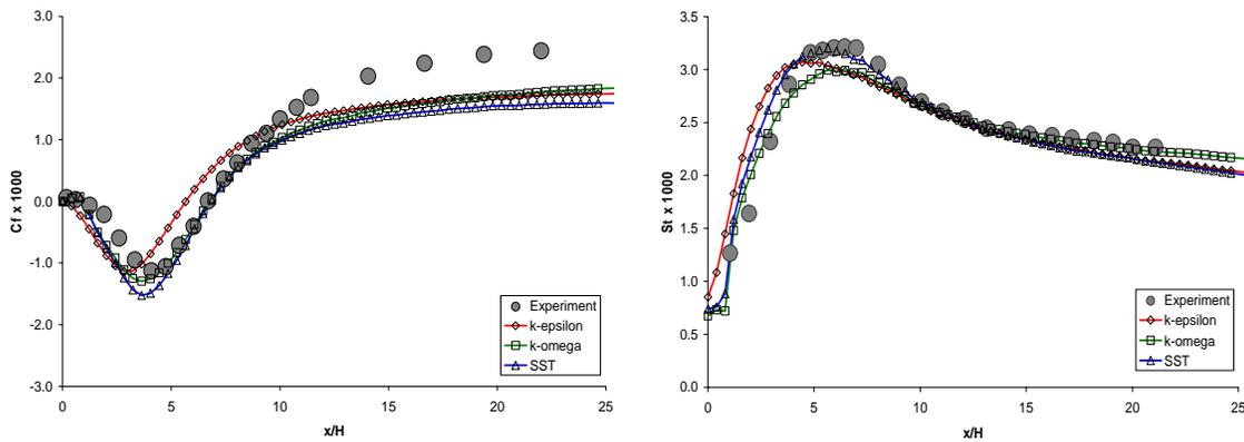
Figure 2 : Comparison of the skin friction coefficient (left) and Stanton number (right) for the  $k-\varepsilon$ ,  $k-\omega$  and SST turbulence model.
