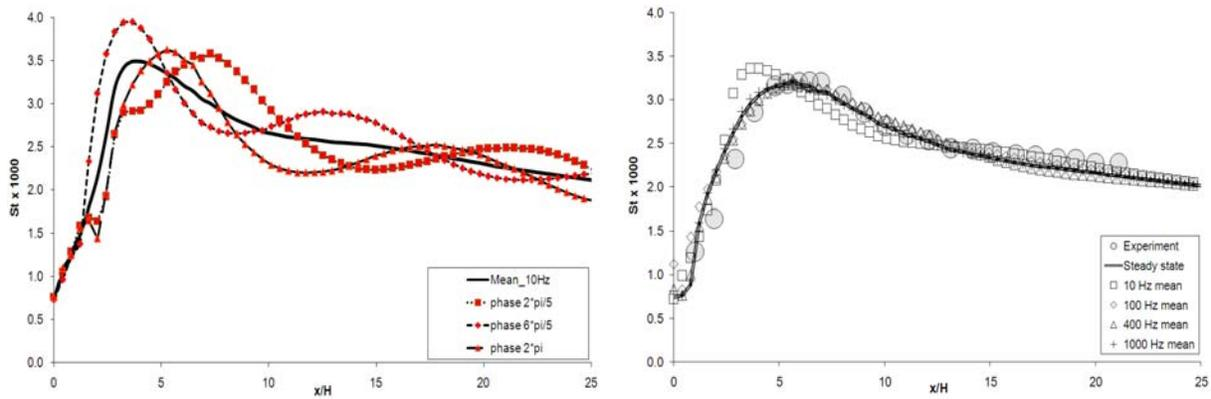
Figure 4: Stanton number: transient (10Hz case - left) and mean (right) results
