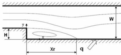
Figure 1: *Geometry and flow configuration for the backward-facing step calculations.*
