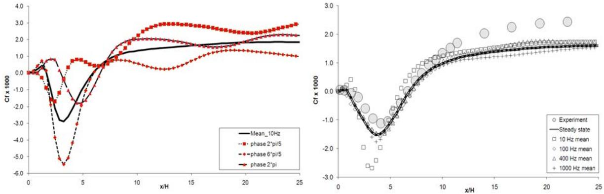
Figure 3: Skin friction coefficient: transient (10 Hz case - left) and mean (right) results
