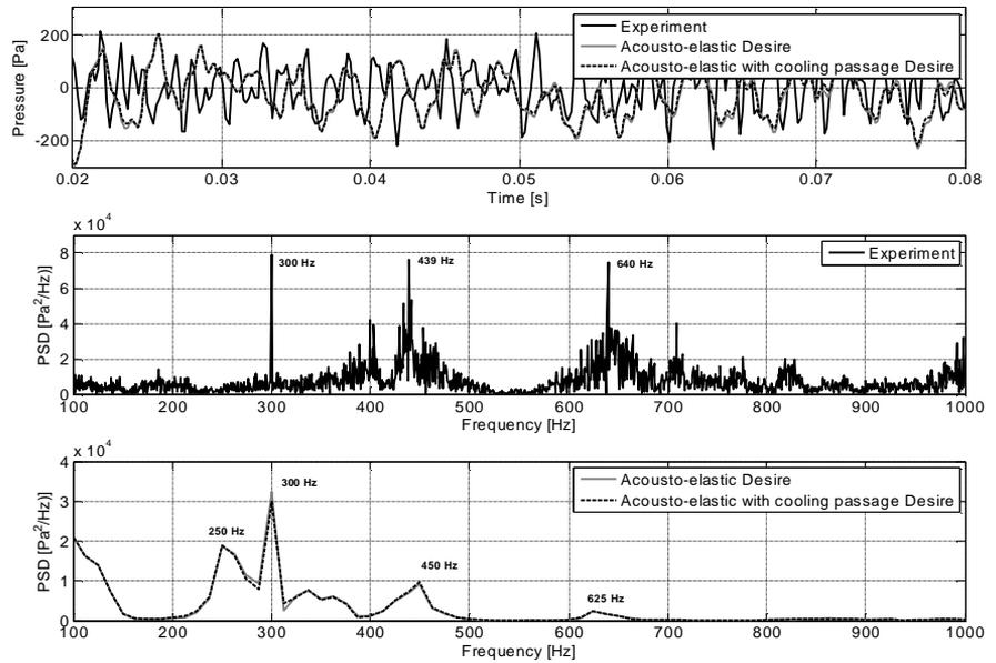
**Figure 7. Comparison of the numerical pressure data with experimental results for the acousto-elastic analysis**
