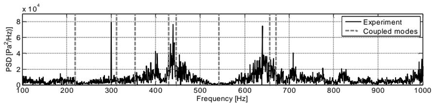
**Figure 18. Comparison of the experimental results of pressure with data from modal analysis**
