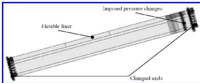
**Figure 6. Numerical acousto-elastic model with boundary conditions (for better visibility the cooling passage is not included)**
