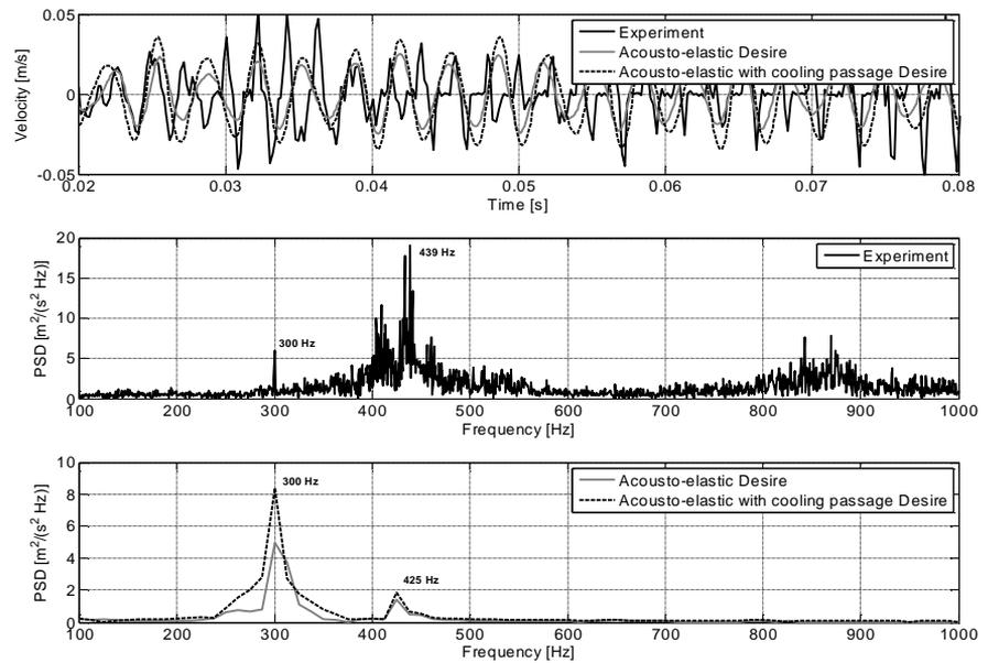
**Figure 8. Comparison of the numerical velocity with the velocity obtained during the experiment**
