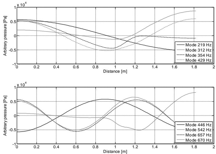
**Figure 16. Selected coupled modes (pressure distribution pattern along centreline)**
