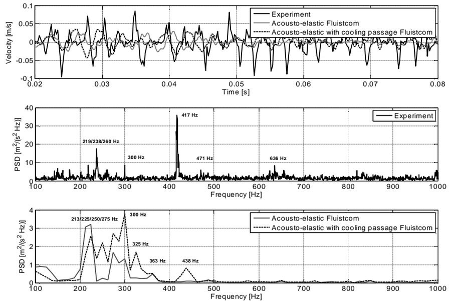
**Figure 12. Comparison of the numerical velocity data with experimental results for Fluistcom liner configuration**
