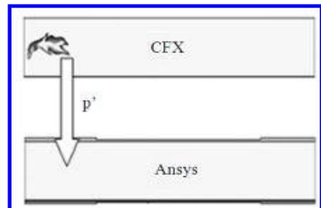
**Figure 3. Data transfer from CFD to FEM code**
