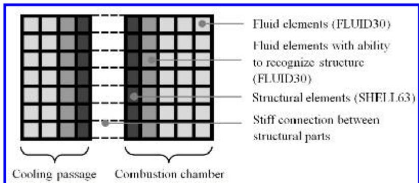
**Figure 5. Transverse cross-section of the acousto-elastic model**
