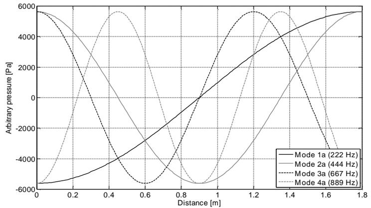
Figure 15. Acoustic modes (pressure distribution along centreline)
