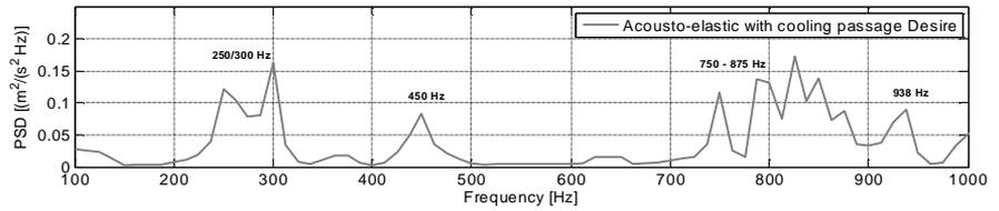
**Figure 10. Velocity spectrum at position of pressure transducer**
