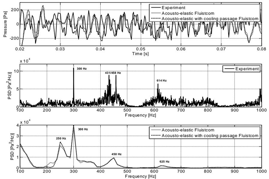
**Figure 11. Comparison of the numerical pressure data with experimental results for Fluiستcom liner configuration**
