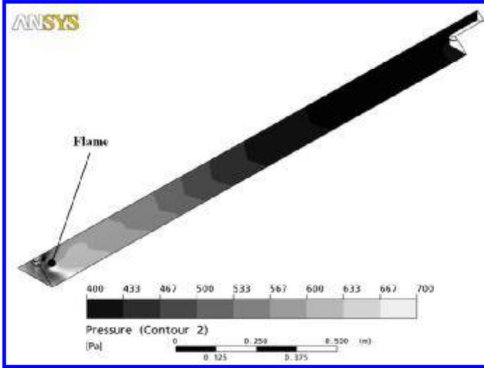
**Figure 2. A pattern of typical pressure distribution inside the combustion chamber (from CFD)**
