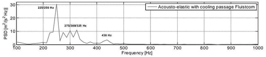
Figure 14: Liner velocity spectrum at location of pressure transducer
