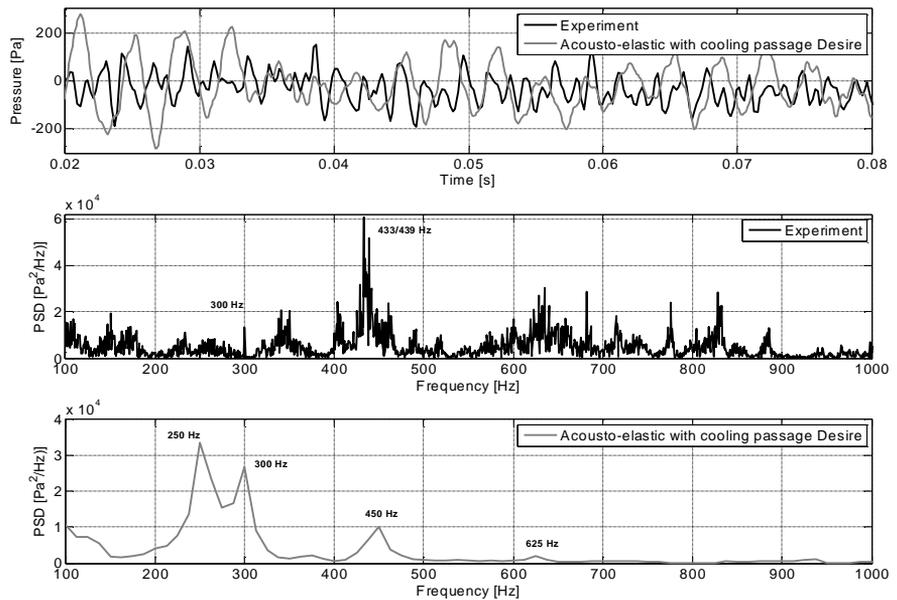
**Figure 9. Experimental and numerical pressure inside the cooling passage**
