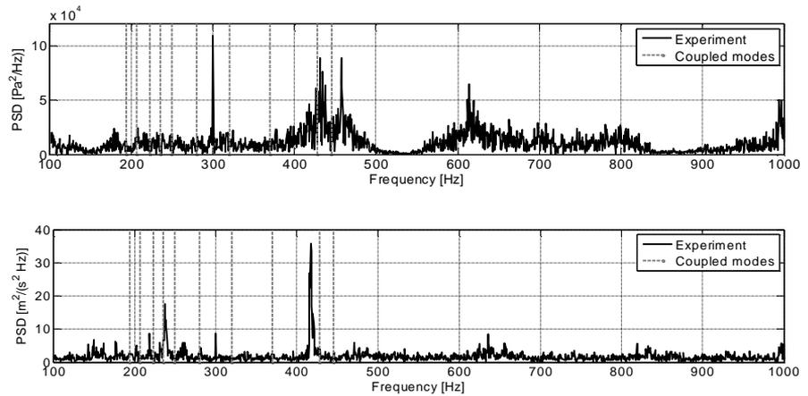
**Figure 21. Acoustic and coupled modes mapped on pressure (top) and velocity (bottom) spectrum**
