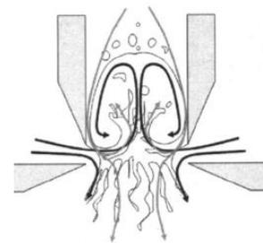
Fig. 1. Flow blurring atomization [1]
