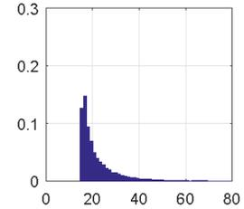
Fig. 3. Droplet size distribution; (x) SMD in  $\mu m$ ; (y) normalized count
