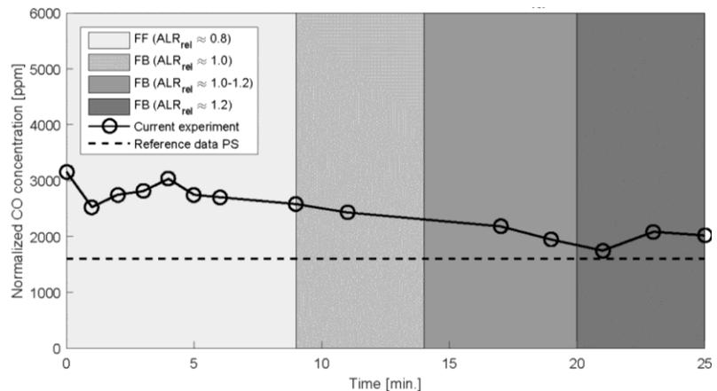
Fig. 4. Normalized ( $15\% O_2$ ) CO emissions in function of atomization regime
