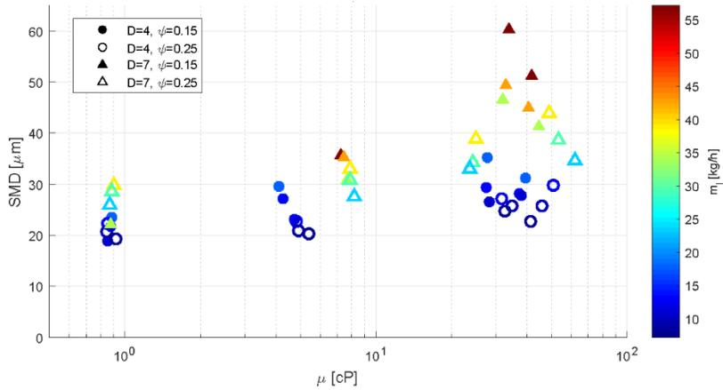
Fig. 2. SMD as a function of viscosity, flow rate and orifice geometrical parameters.
